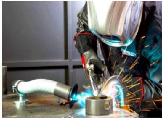
Welder using local exhaust ventilation to remove fume from breathing zone. (Photo courtesy of the Lincoln Electric Company).
